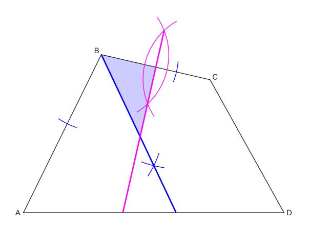
For (a): Scribe two arcs from B using a compass and the same radius. Scribe two arcs of the same radius from the points these arcs cross AB and BC. Draw a straight line from B through the cross where the two second arcs meet.
