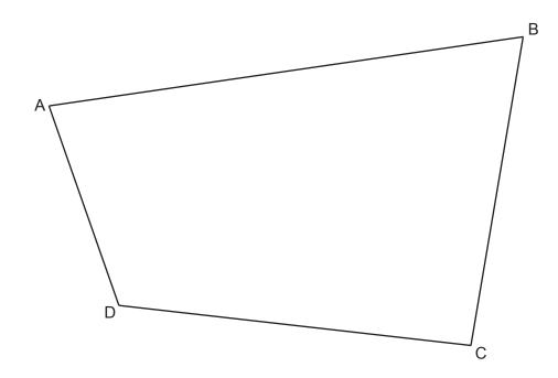
For (a): Construct an angle bisector on angle ABC. Use a compass to scribe two arcs on AB and BC from B which have the same radius. Then scribe an arc from each of the first two arcs with a radius which is greater than half of the distance between the first two arcs. Draw a straight line from B to the cross where the second two arcs meet.
